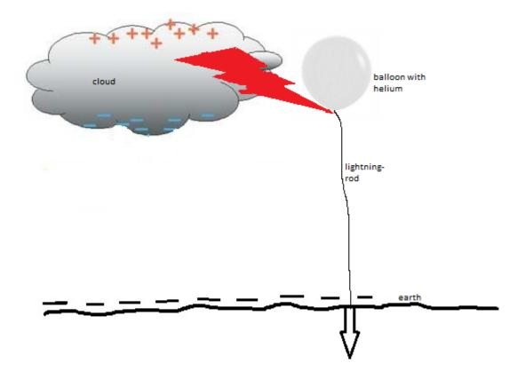
It is known that for the first time in 1750 American scientist, Benjamin Franklin was indicated the only way to guard against lightning. He colud transfered an electric discharge in the atmosphere to ground securely with simple way –metal wire by creating lightning rod and this unique method has not lost its relevance till today..
