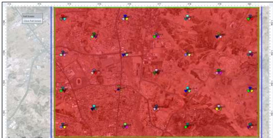
Figure 4. 81: prediction result of Effective Service Area Analysis (DL+UL) in 5G NR technology (After optimization)
