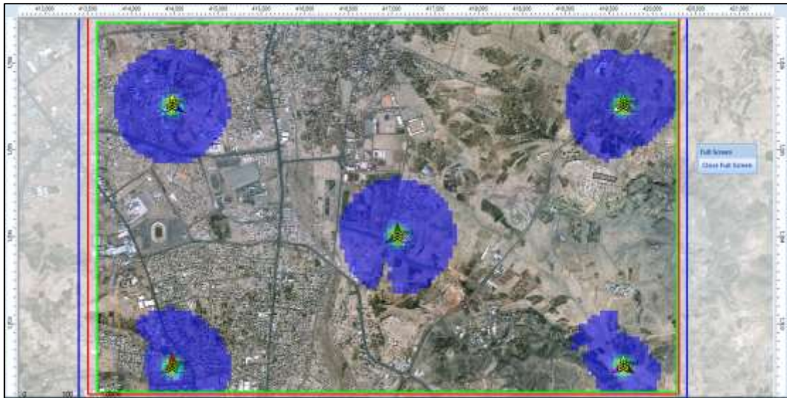
Figure 4.33: prediction result of Coverage by Throughput (UL) in LTE technology (Before optimization)
