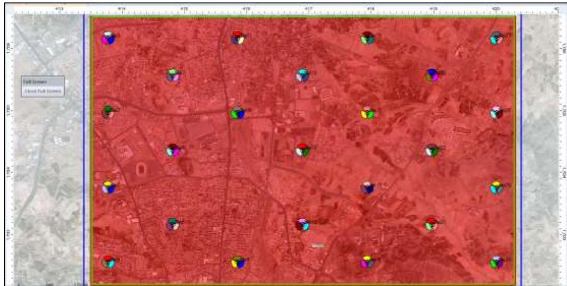
Figure 4. 82: prediction result of Coverage by Throughput (DL) in 5G NR technology (Before optimization)
