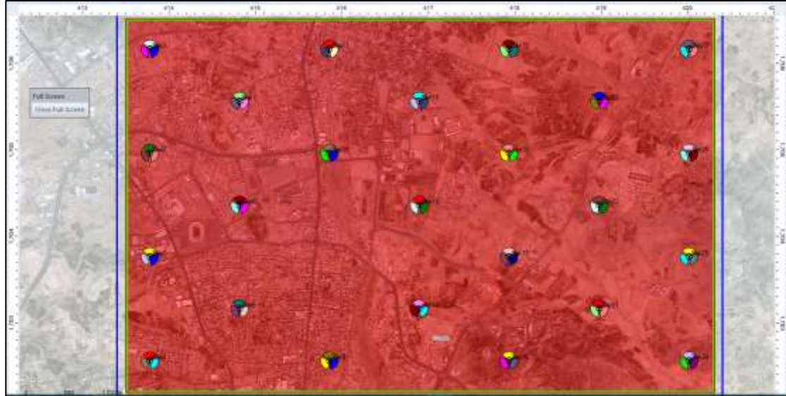
Figure 3. 68: prediction result of Effective Service Area Analysis (DL+UL) in 5G NR technology
