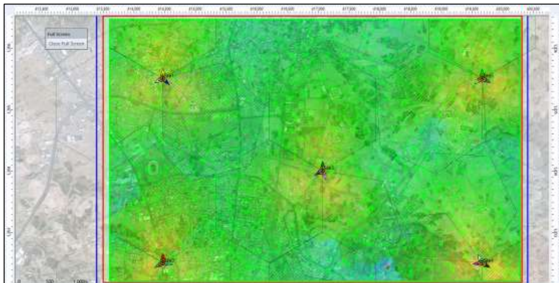
Figure 4. 12: prediction result of Effective Signal Analysis (DL) in LTE technology (After optimization)
