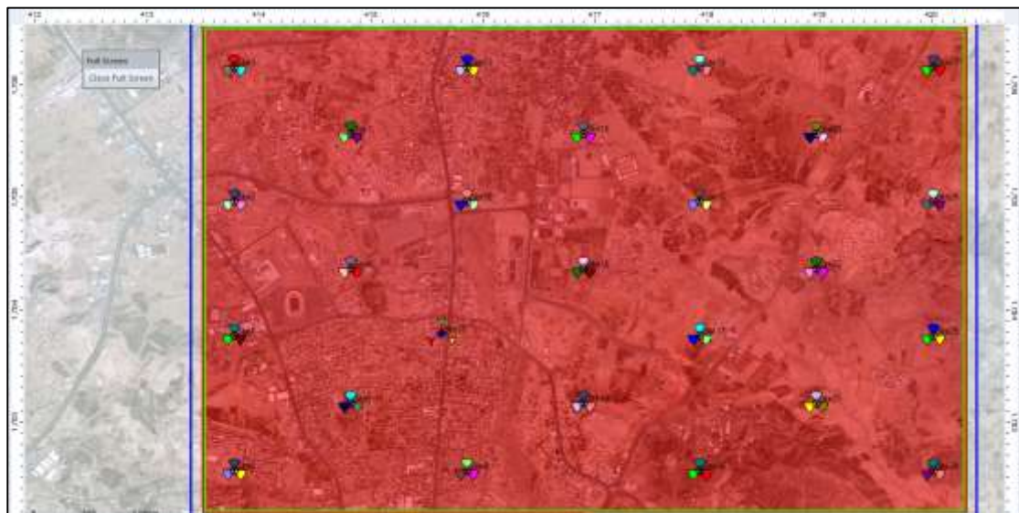
Figure 4. 83: prediction result of Coverage by Throughput (DL) in 5G NR technology (After optimization)
