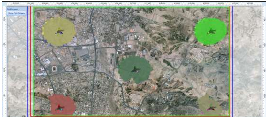
Figure 4. 1: prediction result of Coverage by Transmitter (DL) in LTE technology (Before optimization)
