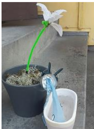
Figure 3. Wind Flower Beam, WFB. Foil arranged as a capacitor and wrapped around an elastic beam becomes a varying resistor at motion.
