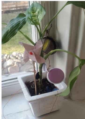
Figure 1. Plant with copper anode, iron cathode, coils and magnets
