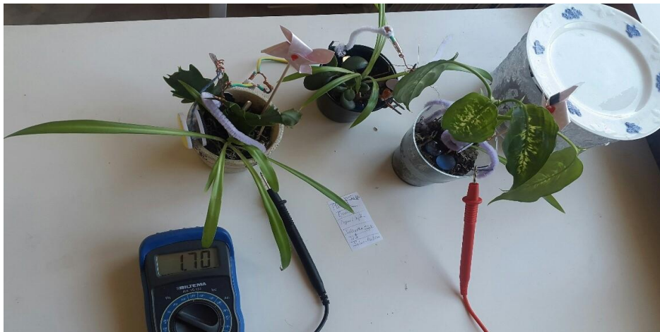
Figure 2. Battery park with 3 pot plants in serial.
