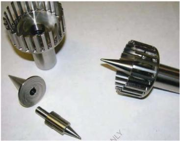
As can be seen in the picture, the dynamic foam generator assembly consists of 3 parts, none of which is movable.
