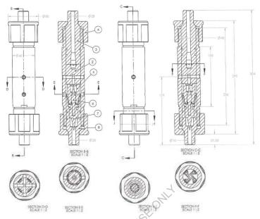
As can be seen from the model and the drawings, the device is designed in such a way that the housing of device 1 (hereinafter all signs according to the model) with internal diameter of 40 millimetres fulfils a very important function of positioning and orienting all elements of the device, which have an external diameter of 40 millimetres;
