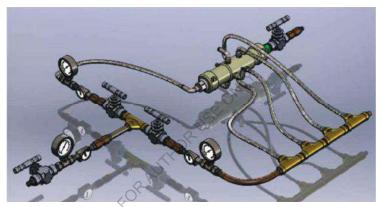
**Figure 3-5**, - The figure also shows a simplified model of a single system level with the additional application of measuring subsystems, - pressure gauges and fluid flow sensors, and also with the use of control valves having both manual and automatic control and adjustment options.
