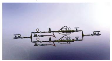
**Figure 2-4**, - the figure also shows the vertical structure of the feeding, metering and on-line preparation system for the various fuel mix options, consisting of a number of independent parts and components with the ability to operate in
