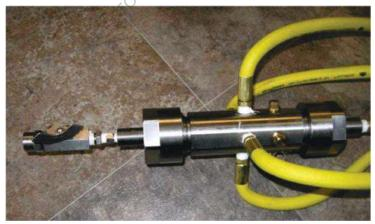
**Figure 4 - 2**, - the figure shows a fragment of the system made in The system is designed to homogenise milk at low pressure (standard systems homogenise at extremely high pressure). In this system the constituent parts are heterogeneous, stainless steel in combination with special reinforced rubber is used as construction material; the reinforcement is made by means of spring steel.
