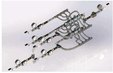
**Figure 2-3**, - the figure also shows a three-dimensional version of the design in which there are two independent supersystems, each with distribution pipework, linked by local supersystems for fluid entry and distribution to levels and a supersystem for connecting two fluid flows from levels, with identical subsystems in each supersystem - valve, gauge, fluid flow sensor and connection pipework fittings.
