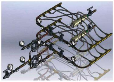
**Figure 2-1**, - the figure also shows a three-dimensional model of the feeding, metering and on-line preparation system for various fuel mix variants, consisting of a number of independent parts and components with the ability to operate in automatic mode, either as a set or singly.
