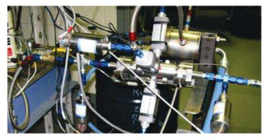
Application of a device with a working diameter of 25 mm and a capacity of 250 litres per hour in the preparation of a gasified fuel composite (from No. 2 diesel and compressed air).
