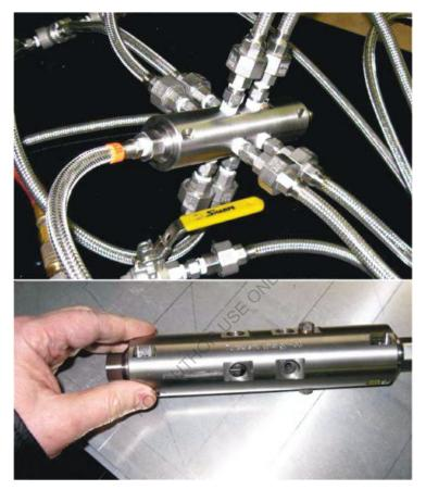
The device is extremely small, allowing its integration without any significant modifications to the fuel system of the thermodynamic equipment.
