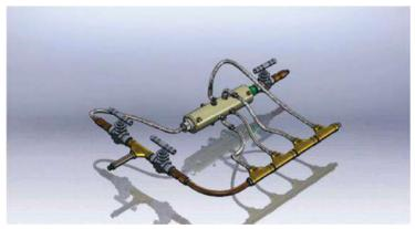
**Figure 3-2**, - The figure shows a simplified model of a single level system without measuring subsystems - pressure gauges and flow sensors, using only control valves with both manual and automatic control and adjustment options.
