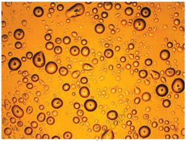
Figure 20 -1. - Figure shows a photo of an emulsion consisting of 20% methanol and 80% diesel #2.
