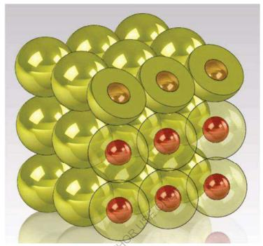
Figure 20-5 also shows the three-dimensional structure of a composite which can be both liquid and solid, e.g. a diamond and copper composite in which each capsule has a core (red in the figure) made of artificial (synthetic diamond) and a shell made of plastic metal - copper, aluminium, nickel, silver, etc.
