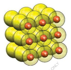
Figure 20 - 3, - The figure shows a three-dimensional model of a composite droplet with transparent shells in which, after injection, nuclei of water (red coloured spheres) explode and in doing so tear the shells of diesel fuel into particles no larger than 1 micron in size.
