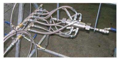
The industrial plant for homogenisation of liquid fuels ranging from diesel fuel No 6 (black oil) to diesel fuel No 2, as well as for micro-minimisation and optimisation of dispersity at the injection of bio-fuels, methanol, ethanol and paraffin from waste plastics, car and other tyres; despite its small size, the plant has the capacity of 1000 litres per hour.
