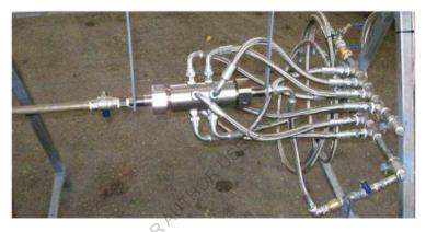
**Figure 4**,-the figure shows a photo of the system for on-line formation of different levels of fuel fluid mixtures or emulsions; the system is made in a homogeneous structure and from one construction material, - stainless steel.
