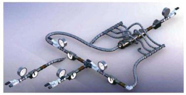
**Figure 3**, - the figure shows a system for mixing, homogenising and, in principle, possible on-line preparation of an emulsion, mainly for fuel fluids.
