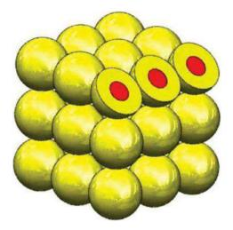
Figure 20 - 4, - The figure shows a three-dimensional model of a composite droplet with opaque shells in which, after injection, nuclei of water (spheres of red in cross-section) explode and in doing so rupture the shells of diesel fuel into particles no larger than 1 micron in size.
