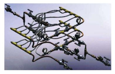
**Figure 2-5**, - In the figure, the distribution systems are highlighted in yellow to convert the linear fluid flows into 4 radial flows.
