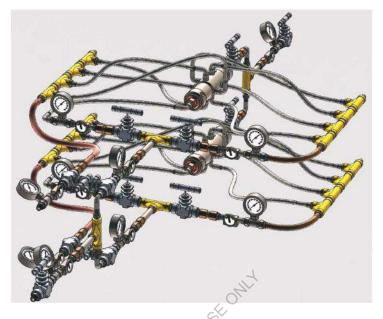
Figure 1, - the figure shows an autonomous online system for blending or emulsion preparation and homogenisation, mainly of liquid fuel materials
