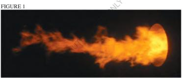
Flame pattern when using normal fuel for this burner - diesel No.4; Fuel flow rate, fuel line pressure, type nozzles, air flow rate, air flow pressure are completely identical for all tests.
