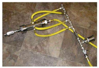
**Figure 4 - 3**, - the figure also shows a fragment of the system made in a nonuniform manner; the system is designed to homogenise milk at a low, - 15 bar pressure (standard systems perform homogenisation at extremely high pressure in the range of 1500 bar).
