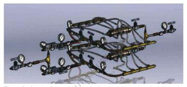
**Figure 2 - 0**, - the figure shows the feeding, metering and on-line preparation system for various fuel mix variants, consisting of a number of independent parts and components with the ability to operate in automatic mode, either as a set or singly.
