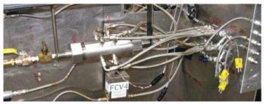
**Figure 4 - 1**, - the figure also shows a photo of the system for on-line and remote formation of various levels of fuel fluid mixtures or emulsions; the system is also capable of on-line homogenisation at the sub-micron level; the system is also made in a homogeneous structure and from a single construction material, stainless steel.
