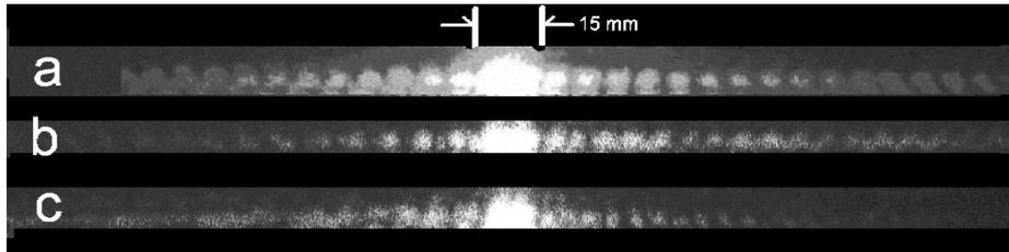
Figure 3: The photographs of the screen images in grayscale for printing: (a) The screen diffraction pattern without the filter. (b) The screen pattern with the filter on the right side of the slit. (c) The screen pattern with the filter on the left side of the slit.
