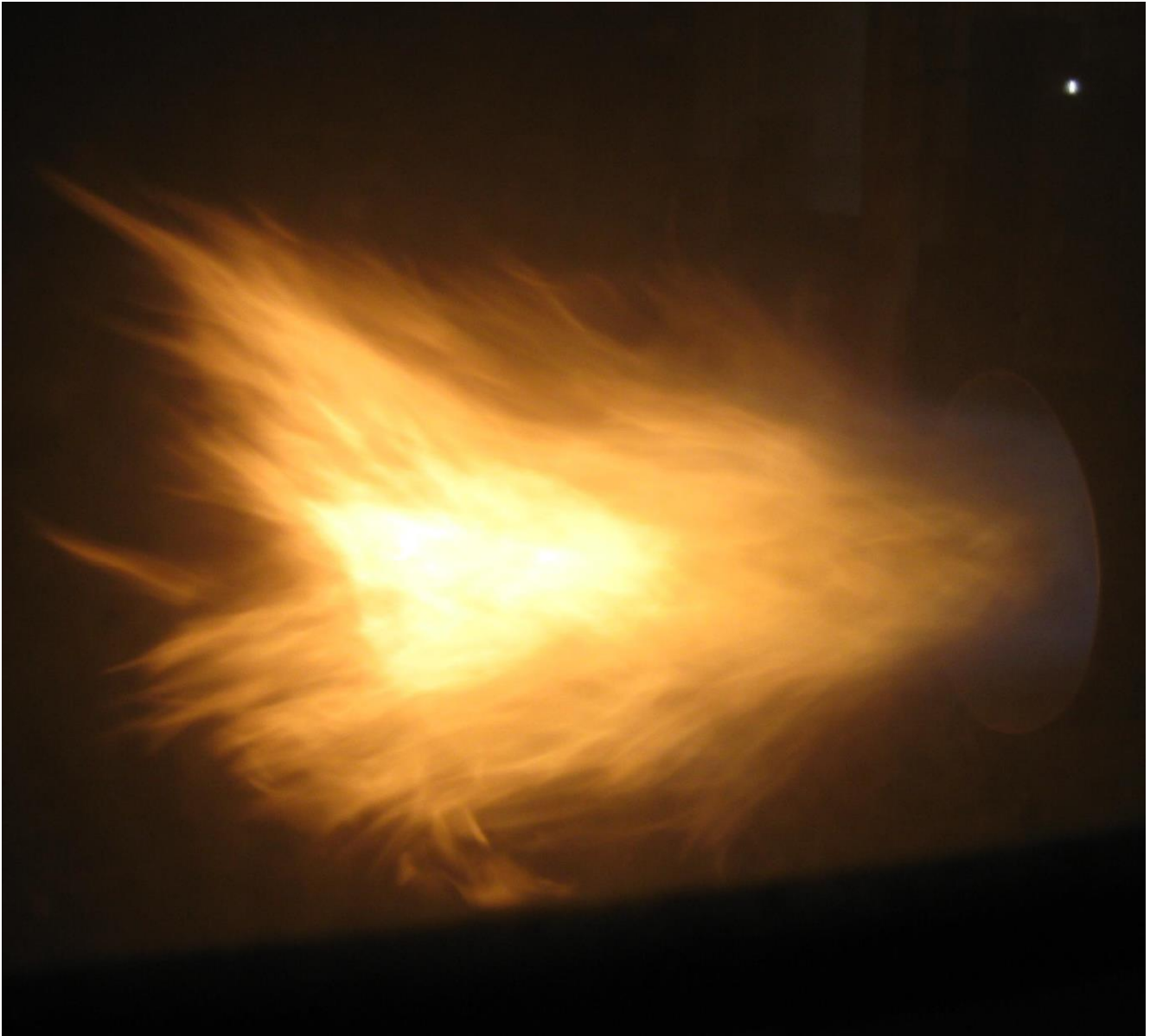
Fig.4. The flame created with the device, connected to burner w/o nozzle is also in a form of vortex tube and the combustion process not require excess air. The CO concentration according with test results is = 0.
