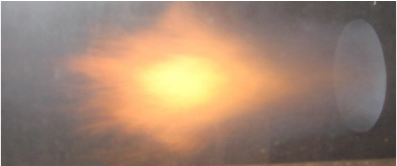
Fig.3. The flame created with the device, connected to burner w/o nozzle is also in a form of vortex tube and the combustion process not require excess air. The CO concentration according with test results is = 0.
