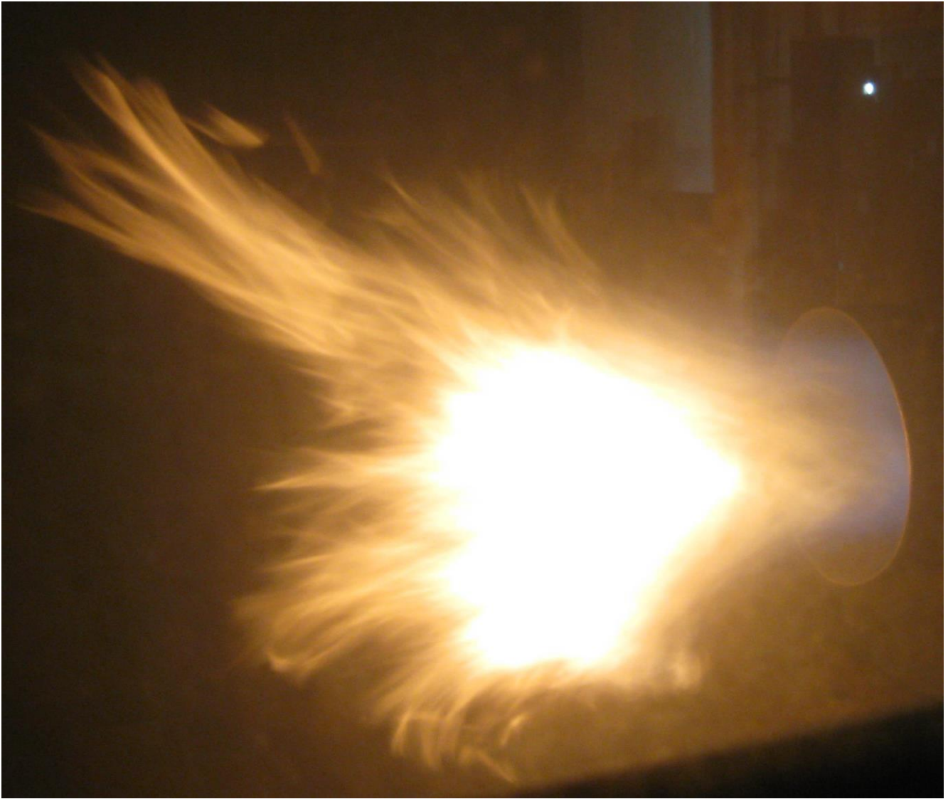
Fig.5. The flame created with the device, connected to burner w/o nozzle is also in a form of vortex tube and the combustion process not require excess air. The CO concentration according with test results is = 0.
