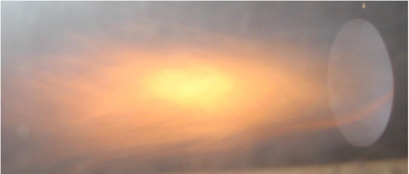
Fig.2. The flame from regular natural gas supply system with a nozzle have a conical shape and the combustion process require at least 20% of excess air. W/o excess air the CO concentration is higher.
