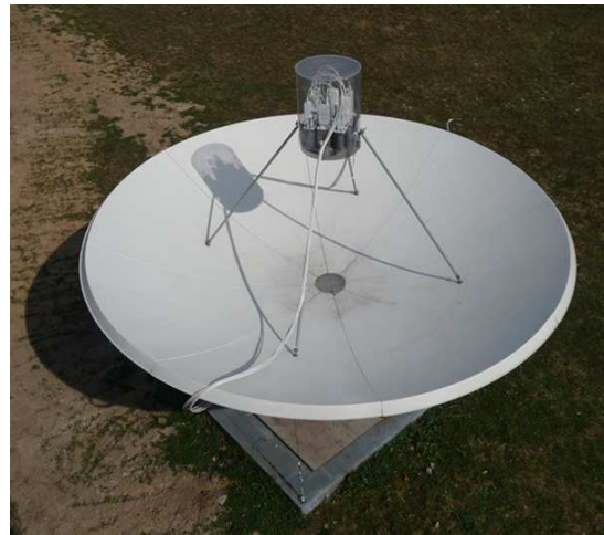
Figure 2: Photo of segmented parabolic dish (Prodelin 1344) of 335 cm diameter and 119 cm focal length. The camera of 9 linearly polarized C band receivers, each consisting of a feed matched to the antenna size and a Norsat 8215F LNB, is supported by four struts.
